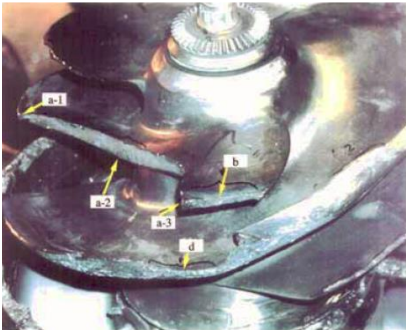
Failure of inducer blade by fatigue
