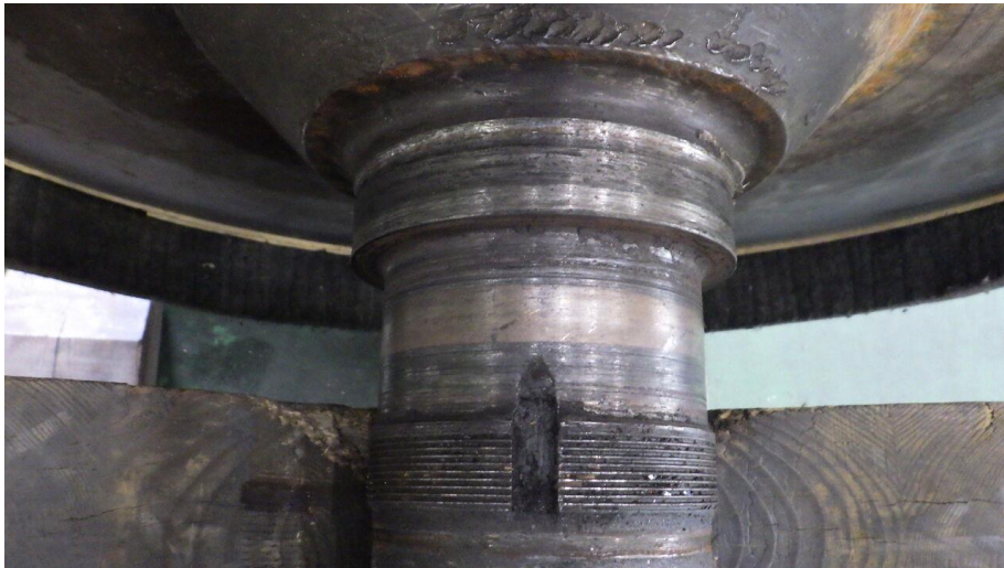
Wear in shaft contacting bearing
